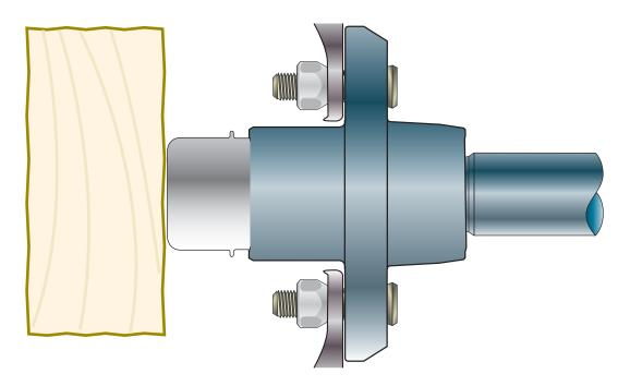
Use a short piece of 2x4 lumber to avoid damaging the dust caps/bearing protector.
