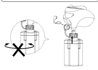
After using battery, please fasten the electrode protection cover, if there is any moisture please dry it before buckling and storing the battery.
