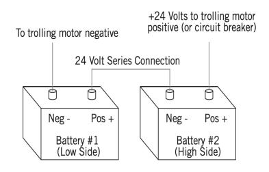
24V connection with two 12V batteries (Figure 1.).
