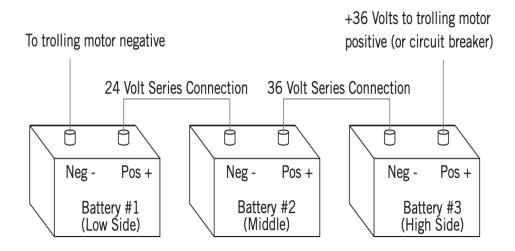
36V connection with three 12V batteries (Figure 2.)
