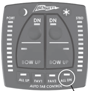
Fully Deploys (Lowers)Both Tabs
