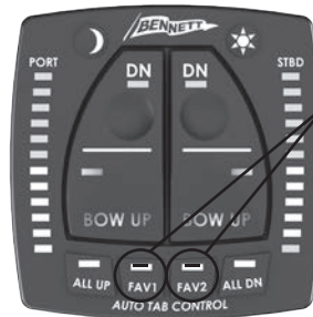
These two LEDs will flash alternately to indicate the system senses rough sea conditions.
