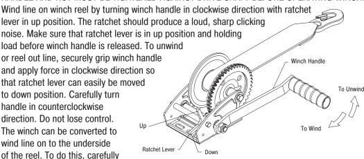
examine ratchet assembly and remove it from winch. Do not lose small parts. Turn the lever over and reassemble. Do not over tighten bolt. Check operation to insure the ratchet lever rotates fully without binding.
