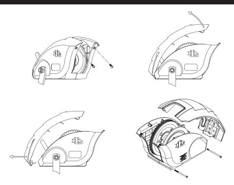
The cover comes off the winch in three pieces. To remove the top cover, loosen and remove the top phillips screws in the front of the cover with a screwdriver. Pull up on the front of the top cover and rotate the top away from the winch. Once the locking tabs are disengaged from the sides, pull the cover straight back to remove.
