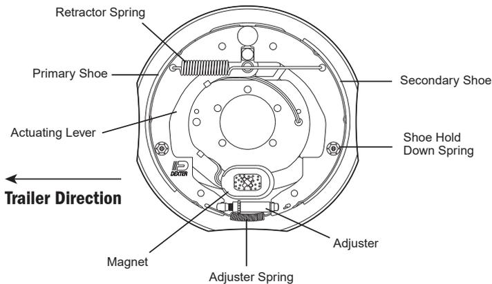
When the electrical current is fed into the system by the controller, it flows through the electromagnets in the brakes. The high capacity electromagnets are energized and are attracted to the rotating armature surface of the drums which moves the actuating levers in the direction that the drums are turning.
