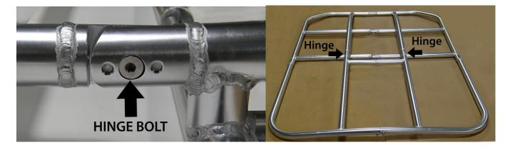
Step 3 - Apply a small amount of grease to fourteen (14) of the Item 7 bolts. Install the bolts into the canopy frame. Only hand tighten the bolts until every bolt is in place and then go back and tighten every bolt.
