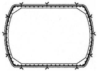
Lace Cover to Canopy Frame: The next step is to lace the cover onto the Canopy Frame. We recommend putting the canvas in place being held by 10 -12 zip ties. Start in the center at the front of the T-Top and tie off the rope to the frame or as shown. Then lace half of the fabric to the center in the back snug but not tight enough to move the fabric. The second half of the lacing will be done tighter to tension the fabric.
