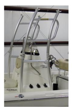
**Install Standoffs on Console:** The next step is to install a standoff on either side of the console. Note the parts of the standoff assembly in the photo below. Look under the console to determine a location suitable for the backing plate shown below avoiding any wiring or obstructions under the center console. **It is acceptable to have the standoff come off the cross bar, front leg or rear leg**. Try and get the standoff as high as possible.
