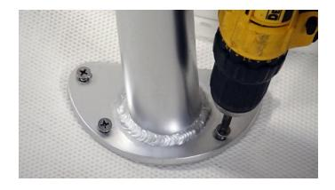
Remove the Top Section Frame to Complete the Standoff Installation: Once the bases are partially screwed into the deck of the boat remove the Four (4) upper leg clamps and the Canopy Frame as shown below. The reason for this is moving the clamps on the top section frame during alignment will scratch the finish of the aluminum. This also allows the legs to be more accurately aligned vertically.
