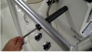
Complete the first standoff installation <u>using Loctite</u> tightening both the Acorn Nut and Backing Plate Nut.
