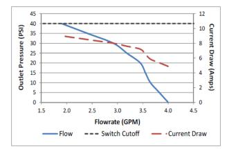
Representative curve of unit operated at nominal voltage Performance will vary somewhat unit to unit Switch cut-off represents the point on the flowcurve at which the integrated pressure switch will turn off the pump
