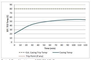
Tested @ ambient temp of 70F (21.1C) @ max run pressure
