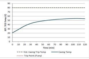
Tested @ ambient temp of 70F (21.1C) @ max run pressure Trip point shown is casing temp at time of TCO trip If there is concern about the ability of the pump to run continuously for long periods of time then in-application testing is highly recommended.
