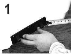
Choose The Location: Preferably inside the chine. You don't want any part of the tab any closer than 10" to the centerline of the boat. Align the bottom of the hinge flush with the bottom of
