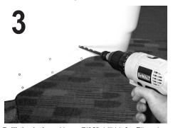
**Drill the holes:** Use a 7/32" drill bit for Fiberglass transoms and a 3/16" drill bit for aluminum and wood transoms.
