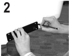
Mark Mounting Holes: Use the hinge as a template. Make sure that you can mount the hinge in the same location on both sides of the boat.
