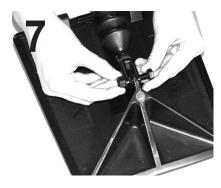
Attach the Actuator: Use the 5/16" nylon bolt and nut (hand tight & snug) to attach the bottom of the actuator to the trim plate in hole #3 (medium pressure).
