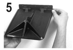
Attach the Plate: Align the plate & hinge holes, and use the 3/8" diameter 'bolts & nuts to secure the plate to the hinge. Hand tighten the nuts as over tightening will create bending.
