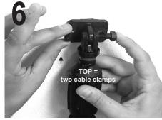
Attach the transom bracket: Use the 5/16x1" #NMS516 Nylon bolt to attach the transom bracket to the TOP of the Actuator (two cable clamps). Secure the Nylon bolt with the 5/16" nylon nut #HLN51618NB.
