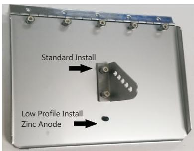
**Attach the Plate Bracket:** Align the bracket from Bag "B" onto the trim plate using the 2 holes closest to the hinge. The third hole is for a zinc anode or if you have height clearance issues you can move the bracket to these holes and this will give you 2.5" less height clearance.
