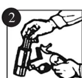
STEP 2 - AFTER SIGHTING POTENTIAL RESCUE VESSEL: Break launcher barrel open, insert Orion 12-Gauge aerial flare and close launcher!
