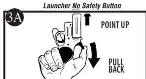
STEP 3A - PREPARING TO FIRE - HOW TO COCK HAMMER With fingers off trigger, hold launcher above head with barrel pointed up, pull hammer back until it cocks (locks in place).
