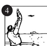
STEP 4 - LAUNCHING/FIRING FLARE Verify launcher barrel is pointed up (as in picture above). Place finger on trigger and squeeze to fire flare. Repeat with second signal.
