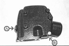
B. Locate four 1/4 inch brass plugs and two 1 inch Iron plugs. Tape each plug appropriately with teflon tape. Securely screw in the 1/4 inch plugs into the threaded holes located at the rear and sides of each elbow, position B (2 per elbow). Securely screw in the remaining 1 inch plugs into each threaded hole at the front of each elbow, position A.
