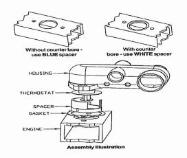
B. Place the thermostat in the thermostat housing (make certain the pointed end faces up into the thermostat housing). Install the appropriate thermoplastic spacer behind it to hold it in place. Reference the illustration at left to determine whether the blue or white spacer should be used. Coat both sides of the thermostat housing gasket (with continuity rivets) with an appropriate sealer (part # 18-9070) and position gasket onto the intake manifold.
