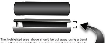
The highlighted area above should be cut away using a band saw. If this is not available, contact your local machine shop to perform the task. The section, when removed, should be between .3150 inch to .3250 inch wide.
