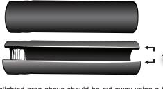
The highlighted area above should be cut away using a band saw. If this is not available, contact your local machine shop to perform the task. The section, when removed, should be between .3150 inch to .3250 inch wide.
