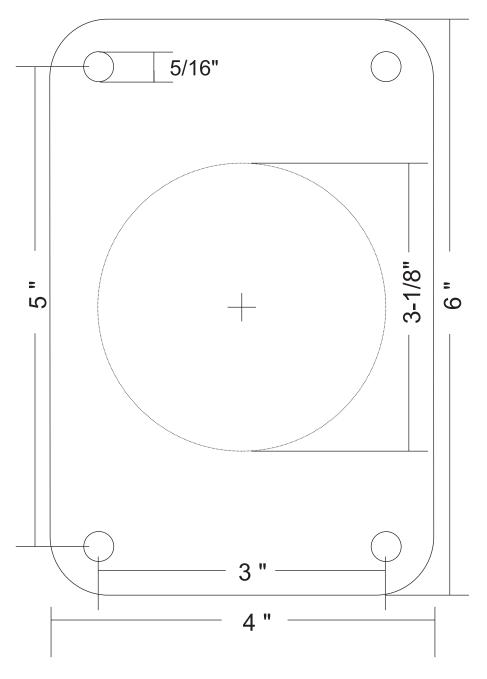
Please print at 100 percent for accurate sizing. Slight scaling may still occur. Therefore, before drilling, it is recommended that all template dimensions be measured for accuracy.
