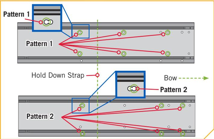
**NOTICE:** If Pattern 2 is used, the right side plate must be removed to access the mounting holes in the base of the Mount.
