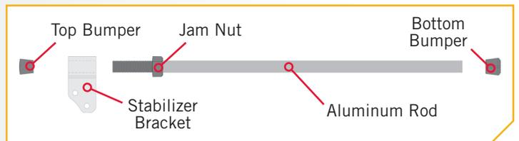
**NOTICE:** The Bow-Mount Stabilizer Bracket can be installed on the left or right side of the Steering Module. When mounting the bracket onto the Ultrex, the two Nylock Nuts (Item #16) are discarded because the bolts are secured directly into the Steering Module.
