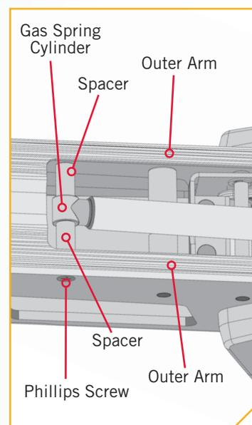
**NOTICE:** Screws have a pre-applied thread locker. DO NOT apply additional thread-locker to the screws as it may prevent future removal.
