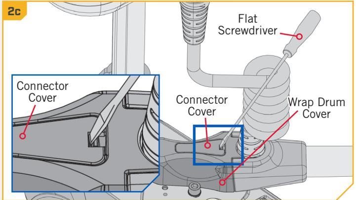
**NOTICE:** Please note the orientation and routing of the plug and wires for re-installation.
