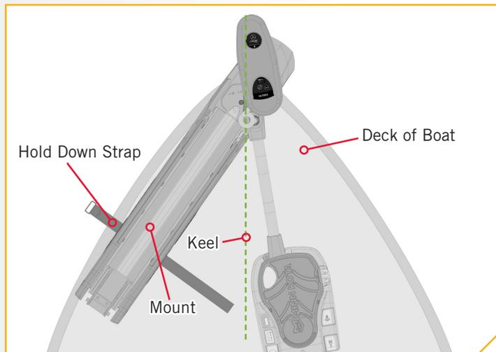
**NOTICE:** This motor weighs approximately 55 lbs. We recommend having a second person help with the installation.
