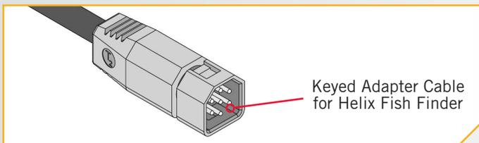
**NOTICE:** The connectors are keyed to prevent reversed installation.
