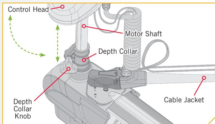
**NOTICE:** After the cable(s) exit(s) the Coil Cord, it/they should be routed through an established routing system on the boat, in an area with minimal interference. Power cables or other elements that may produce interference for the sonar signals. Inspect the selected route carefully to ensure that there are no sharp edges, obstacles, or obstructions that may damage the cables.
