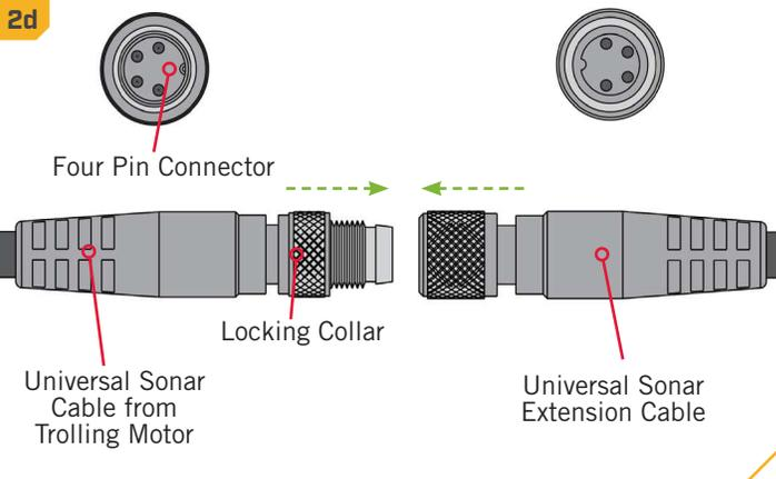
**NOTICE:** The connectors are keyed to prevent reversed installation.
