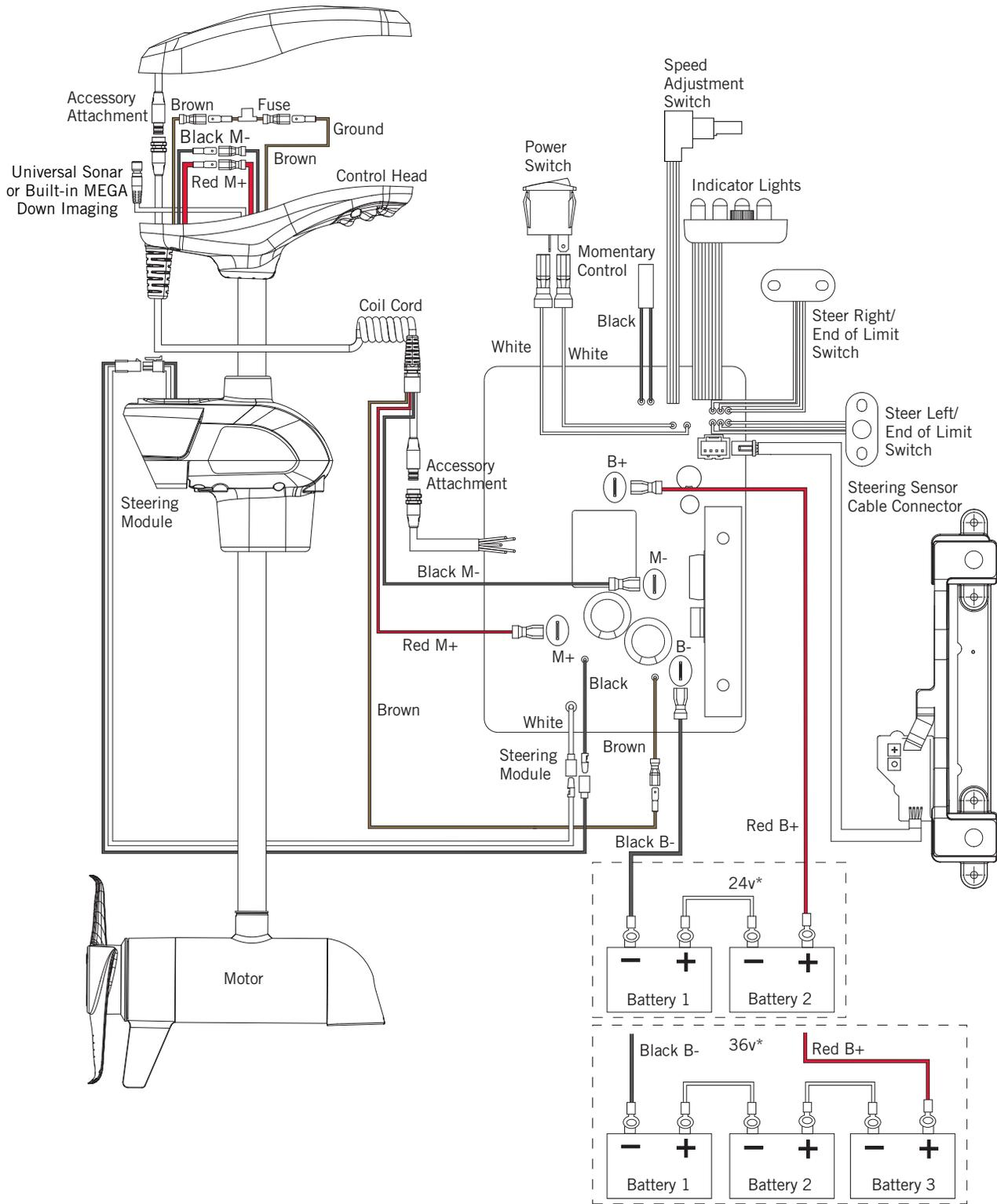
**NOTICE:** This is a multi-voltage diagram. Double-check your motor's voltage for proper connections. Over-Current Protection Devices are not shown in this illustration.
