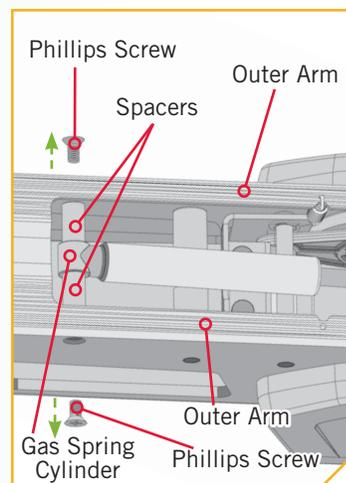
**NOTICE:** Use a #3 Philips screwdriver to remove the screws. They have a pre-applied thread locker. Not using the recommended tool can cause damage and prevent them from being removed.
